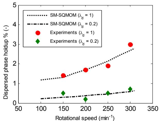
Figure 1. Comparison between the simulated and experimental dispersed phase hold up.
