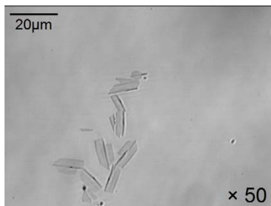
Figure 4. Microscopic image of the interfacial self-aggregates of ZnTPyP transferred on a cover glass after a CLM measurement ( [\text{ZnTPyP}]_0 = 2.5 \times 10^{-6} M).
